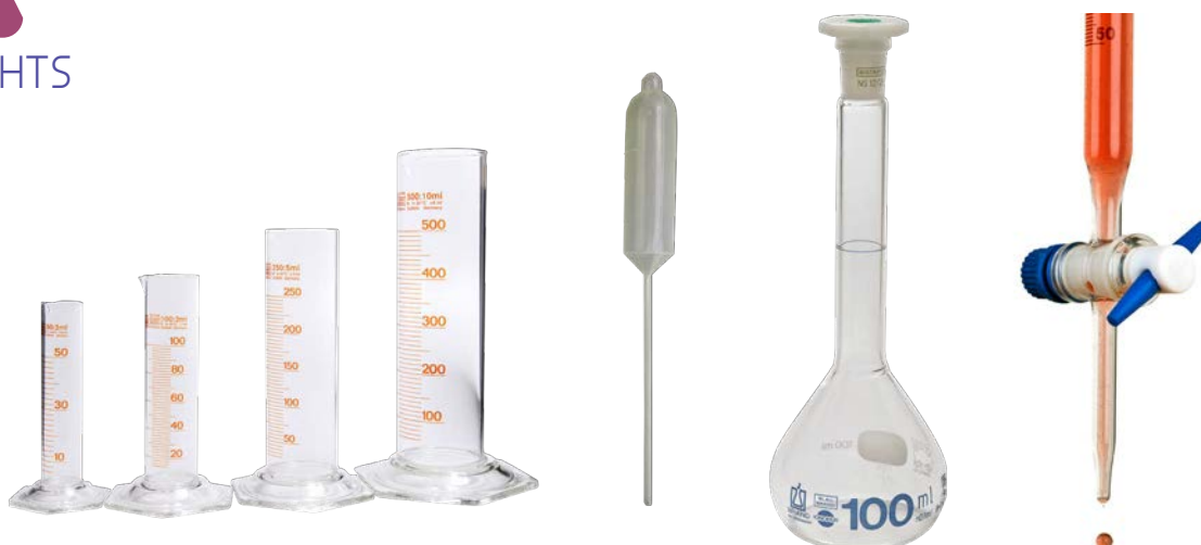
Left to right: graduated cylinders, pipet, and volumetric flask, and buret (not to scale).
