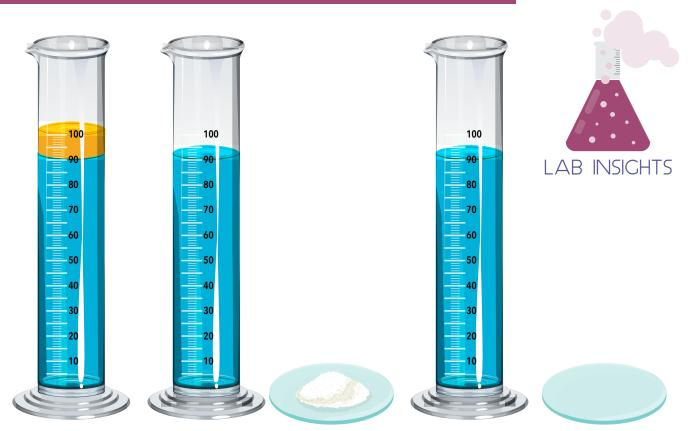
The oil is 10 percent of the total liquid in the graduated cylinder, and the oil is not soluble in the water.
