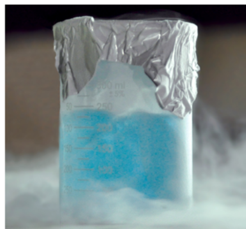
This beaker contains oxygen that is so cold it is in its liquid phase.
