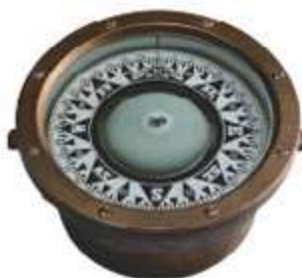
4-7 This compass rose shows the cardinal and intercardinal directions, as well as degrees.
