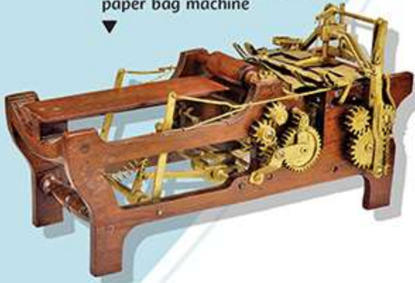
Model of Margaret Knight's paper bag machine
