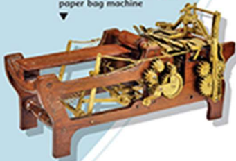
Model of Margaret Knight's paper bag machine
