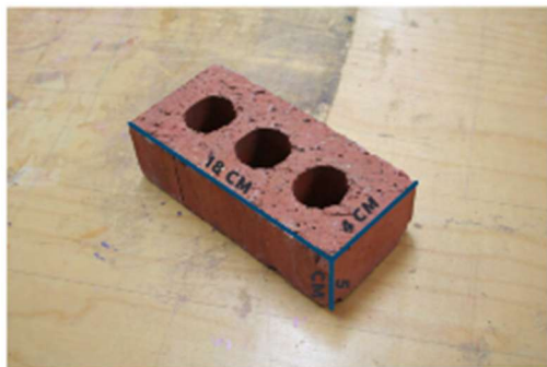
By multiplying these 3 dimensions, we can figure out the volume: 18 \text{ cm} \times 5 \text{ cm} \times 4 \text{ cm} = 360 \text{ cm}^3 .
